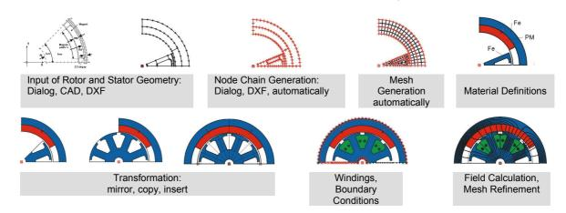
Additional to simple field calculations are also multiple calculations possible. Thereby field calculations can be automatically operated for arbitrary currents in the windings and for different positions of the rotor. For every position magnetic field, torque, forces, winding fluxes and voltages are calculated. Out of that engine models are deducted und characteristic curves determined for linear or rotating machines with excitation by permanent magnets or current and for induction machines.
